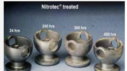
Application: Nitrotec treated Swivel Hubs – after 20 times longer in the test.
